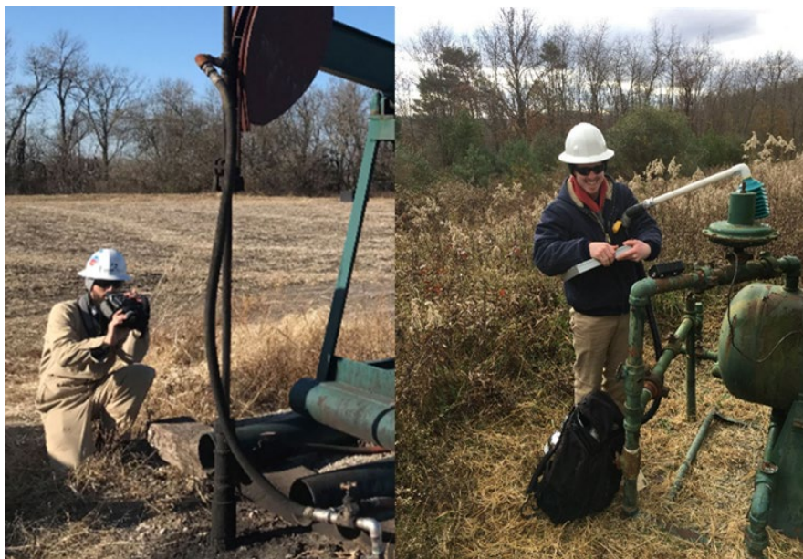
Figure 4. Emissions were identified using optical gas imaging (OGI) and quantified using the BHFS.
